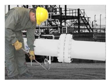
Clean clogged bleeder, vent and instrument tap valves safely and efficiently while containing process material.
