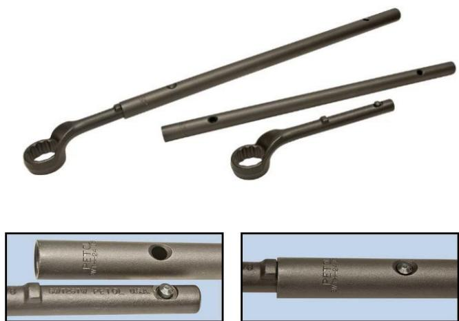
The PETOL® Tube Handle Wrench is a 12-point offset box end wrench that can be used with or without a detachable tube handle. The tube handle **provides additional torque** when tightening or breaking loose nuts. Handles are held in place with a spring-loaded locking button
