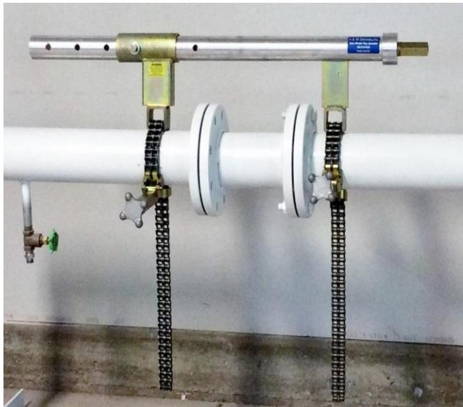
Ideally suited for spreading lap joint, slip on, or flat face flanges.
