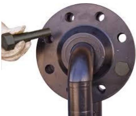
\*Correct size pin will match the Bolt-HOLE size of your flange\*
